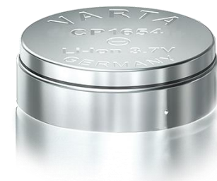
Rechargeable lithium-ion coin cell for premium wearable devices
